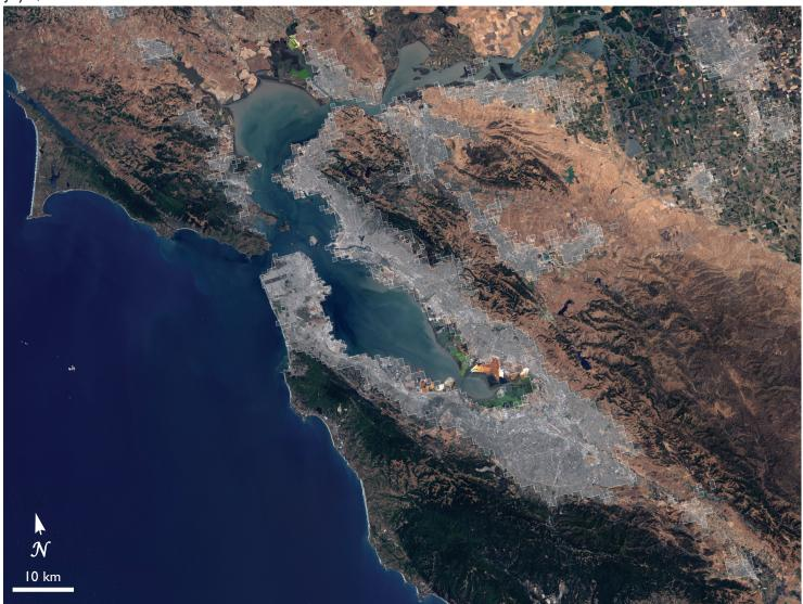
Satellite image of the San Francisco Bay area on July 7, 1999. Vegetation appears green, water blue, and bare land tan. (Data from the ETM+ instrument, bands 7 [infrared], 4 [near-infrared], and 2 [green], on the Landsat 7 satellite.)
