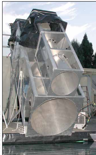
The Aquarius instrument prototype was used to test the mission's measurement principle by observing how 1.413 gigahertz microwave emissions responded to changes in salinity in a salt-water test pond.
