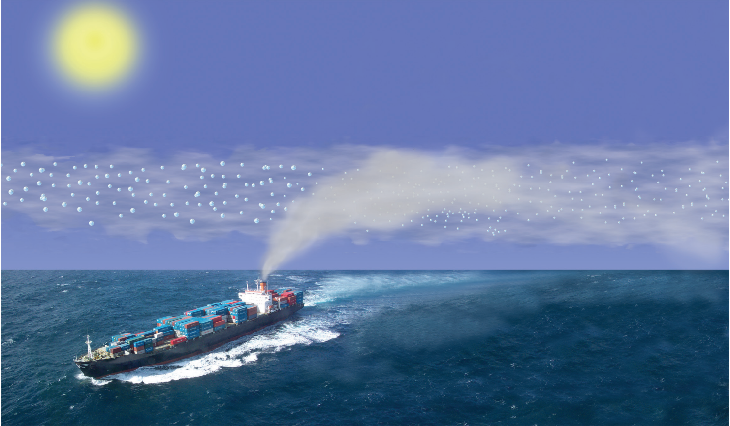
Schematic illustration of the effect of cloud nucleation particles from ship exhaust resulting in a larger number of cloud droplets in a given volume of cloud but with smaller droplet sizes.
