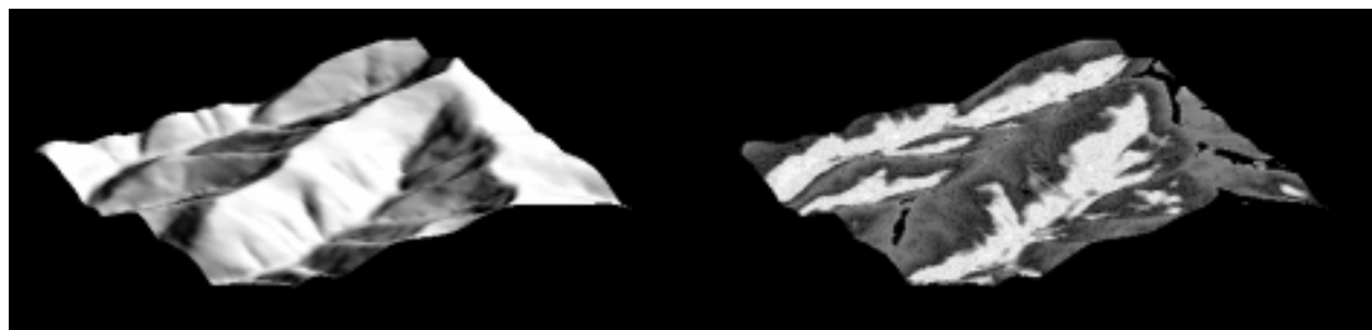
Figure D-1. Total radiance (radiosity) emitted from an isothermal homogeneous scene ( \epsilon=0.9 ), consisting of directly emitted and multiple-scattered components. Left: Digital elevation model "illuminated" by sun at lower right, assuming a Lambertian surface of uniform reflectivity. Right: Multiple-scattered TIR component, contoured with black = 0-1%, gray = 1-3%, and white = 3-5% of the direct emitted component. Perspective view calculated from a 7.5' DTM having horizontal resolution of 30 m. Subscene is 3 km across.
