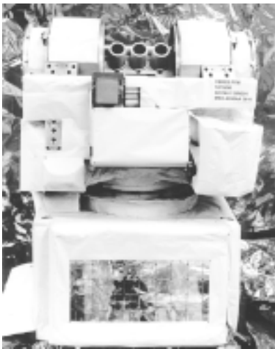
◀ This is a photograph of the Clouds and the Earth's Radiant Energy System (CERES) instrument. CERES measures both solar-reflected and Earth-emitted radiation from the top of the atmosphere to the surface. It will also determine cloud properties including the amount, height, thickness, particle size, and phase of clouds using simultaneous measurements by other instruments. One CERES scanner (left) was successfully launched on the TRMM spacecraft on November 27, 1997. Two more CERES scanners will fly on the Terra as well as the EOS PM spacecraft.
