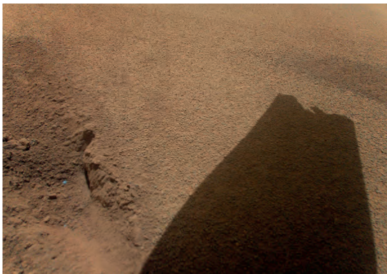
Ingenuity's Last Flight. On January 18, 2024, this image of a damaged rotor blade's shadow confirmed that NASA's Ingenuity Mars Helicopter would fly no more. This tiny tech demo was designed to attempt five flights, the first time an aircraft achieved powered, controlled flight on another planet. Ingenuity surpassed this achievement, completing 72 flights in almost three years of operations, flying 14 times farther than planned as it transitioned from a demo to an aerial scout for NASA's Perseverance Mars rover. Although grounded, Ingenuity will continue to collect data to lead the way for future exploration. Image and text credit: NASA/JPL–Caltech
