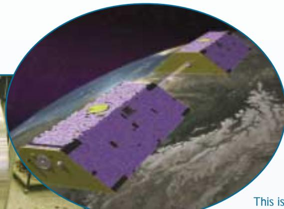
This is a schematic diagram of the two GRACE satellites in orbit with the K-band microwave beam connecting them and precisely tracking fluctuations in the distance between the two satellites. The fluctuations are used to infer changes in the gravitational field on the surface of the Earth below.
