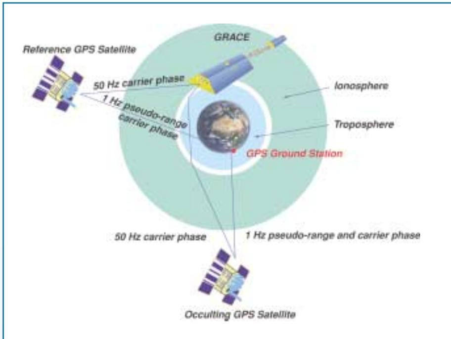
This diagram, originally provided by GFZ, illustrates how the occultation process works. The GRACE satellite tracks a GPS satellite as it "rises" and "sets" through the limb of the atmosphere, while a second GPS serves as a reference point.
