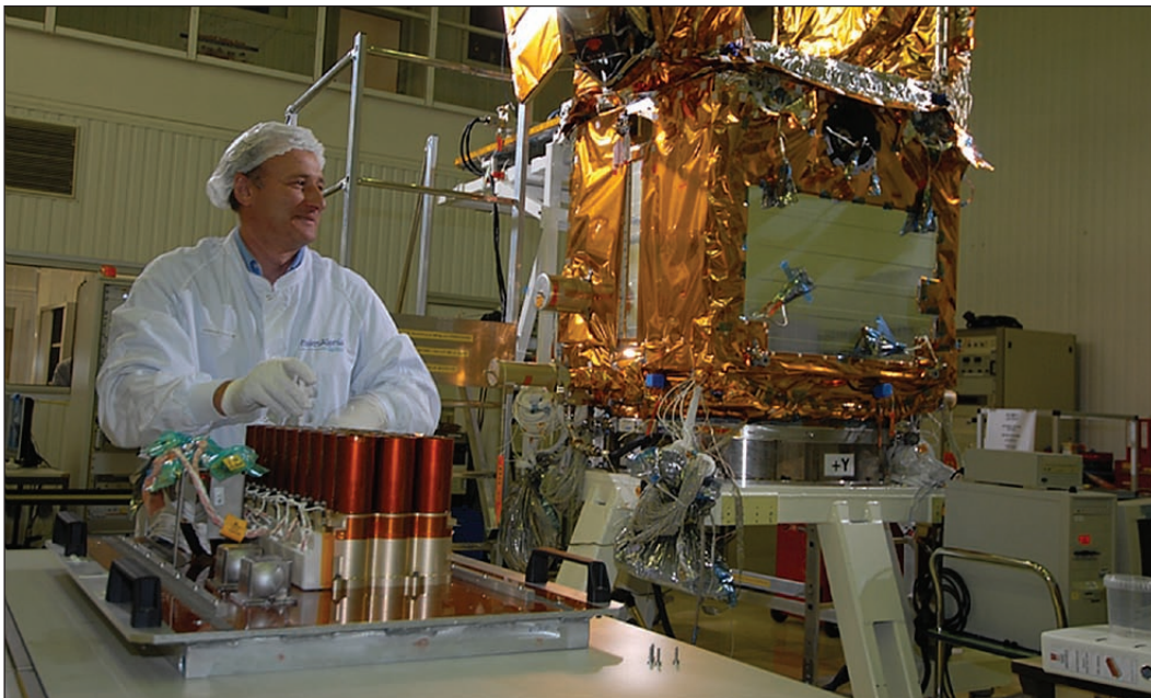
T2L2 is an optical time transfer experiment on Jason-2. Using pulses of light, it allows synchronization of remote clocks on Earth and high-accuracy monitoring of the satellite's clock. Image credit: G. Benjamin, CNES
