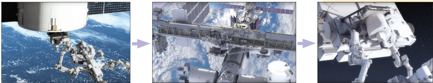
Once the Dragon trunk docks with the space station, the robotic arm will remove the Instrument Payload, followed by the Nadir Viewing Platform and place them on a temporary platform while they move to ELC-4. Once at the correct location, the Nadir Viewing Platform will be attached to ELC-4, followed by the Instrument Payload.
